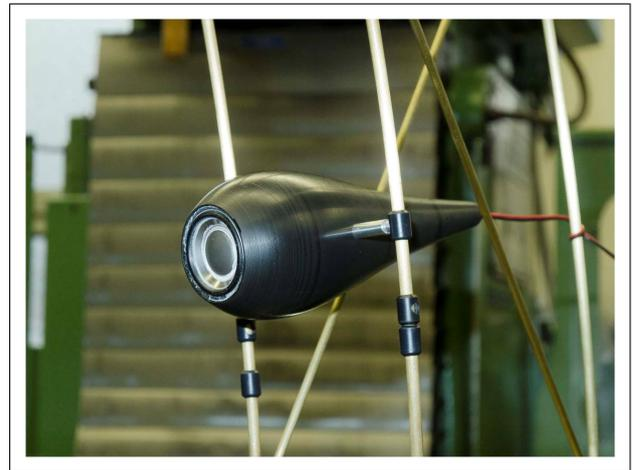
Figure 2. Prototype of the drop-like loudspeaker.
