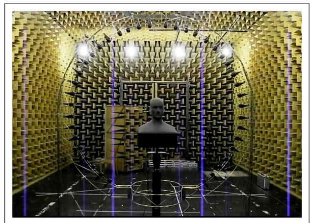
Figure 5. Photo of the HRTF measurement set-up while measuring the HRTFs of a dummy head.
